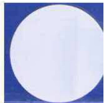
Fig 3: SDI pad of the downstream MMF effluent, with coagulant addition.
