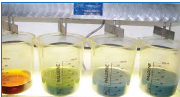
Jar Testing of Chrome Reduction Process
